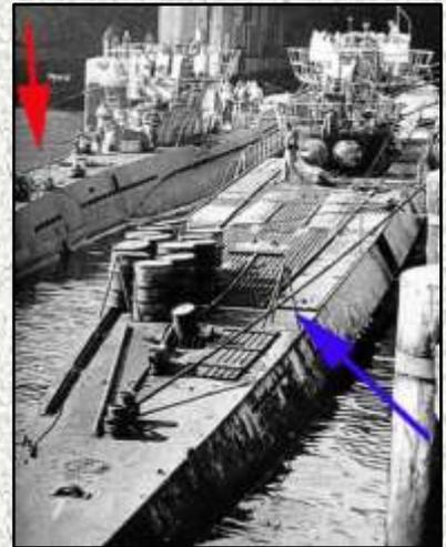
Above (111): The blue arrow points to the rear tripods on the IXD2 U 862 while the red arrow points to the style which faced outwards on the VIIC/41 U 995.
