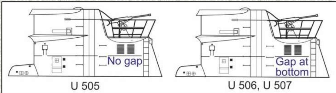
Above (14): As covered earlier, there was a difference in respect to the two grills lower down. On the IXAs, IXBs and the *Deutsche Werft* IXC U 505, there were eight horizontal bars arranged with equal distance between the bars and no gap at the bottom. From U 506 onwards, the number of bars was the same but a significant gap appeared beneath the lowest bar.
