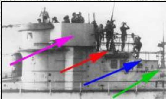
Left (93): U 172 with Turm II in August 1943. The purple arrow points to the radar box, red to the upper platform and green to the lower platform. The blue arrow points to an area at the front of the lower platform in which the sides of the hull were raised to mid-level. These raised sides did not feature on Turm IIs on VIICs.
