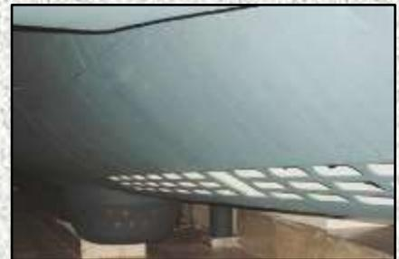
Above (112): The underside of the bow of the museum boat U 505 showing the unpainted hydrophones arranged around the dome-shaped *Balcongerät* device.
