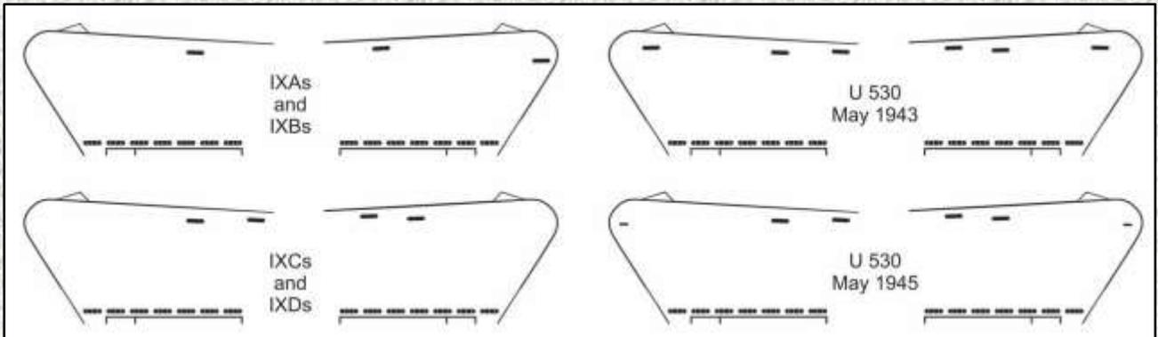
Above (64): A guide to the difference between the bow vents. Note the extra vent on the starboard side of all IXAs and IXBs.
