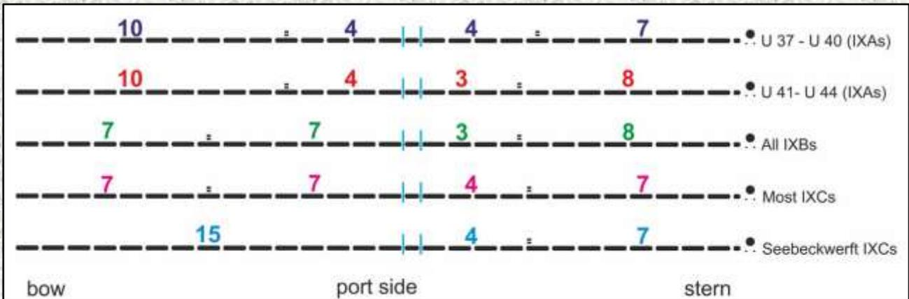
Above (67): The position of the two sets of double footholes on IXAs, IXBs and IXCs.
