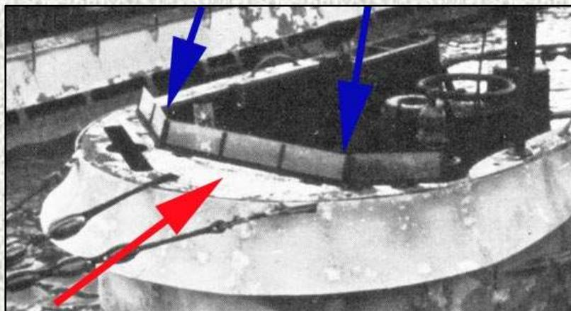
Above (17): The windscreen can clearly be seen on U 160 in December 1942. The red arrow points to the windscreen base plate while the two blue arrows point to the angle between the three sections. We can see that on U 160 the screens were present in three directions: a double screen at the starboard side, a triple screen in the middle and a single screen on the port side.
