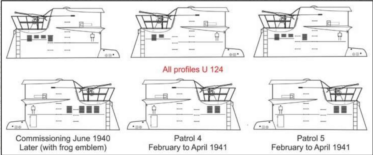
Above (11): These profiles show that grills lower down on U 124 varied greatly. Presumably the grills were easily interchangeable to make their removal or fitting easier. It took time before the Kriegsmarine determined how many grills were required for the Type IXs and this was part of a wider problem that both the IXs and VIIs experienced with air intakes.
