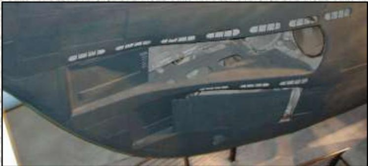
Above (62): A somewhat damaged U 67 in October 1941. While some vents have been lost due to damage to the bow, this boat had port pattern A which was commonplace at the time.
