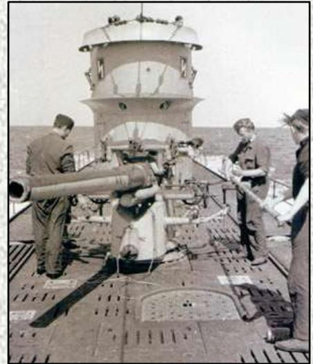
Above (42): The access hatch is clearly offset to port ahead of the 105mm deck gun.
