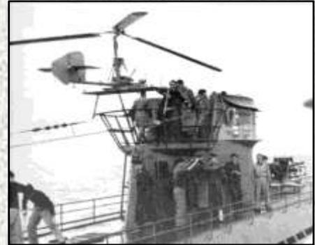
Above (113): A Focke-Achgelis FA 330 *Bachstelze* being tested on U 532 in the autumn of 1942. The IXC has a yellow training band above the spray deflector, indicating that it had not yet been assigned to an operational flotilla.
