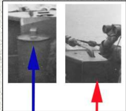
Above (21a-21b): On the left is the IXA U 38, with the blue arrow pointing towards a lid on top of the third periscope. On the right is the same area of the IXB U 103.
