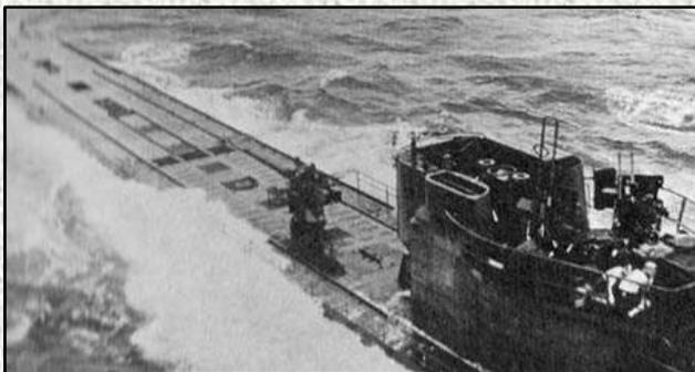
Left (87): In this photo of the IXD2 U 848 in November 1943, we can see the torpedo channels extending way beyond the 105mm deck gun in channels FS and FP.
