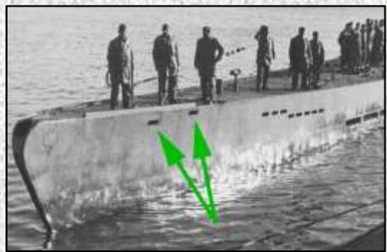
**Footholes** - As can be seen from the drawing below, the key difference is the position of the double footholes. The purpose was presumably for crewmen to put their foot in when moving to a small boat over the side. A modeller converting to an IXA or IXB needs to fill and drill these double footholes.
