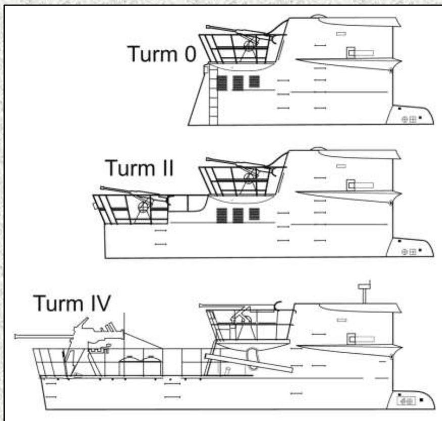
Above (95): To distinguish between a Turm II and Turm IV, we need to look at the upper platform. If there is only one gun then it is a Turm II but two separate gun mounts means it is a Turm IV.
