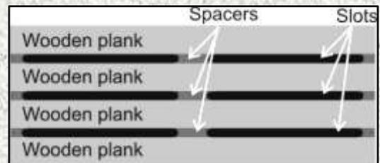
Above (80): The older slotted type of deck which used spacers at equidistant lengths between the planks.
