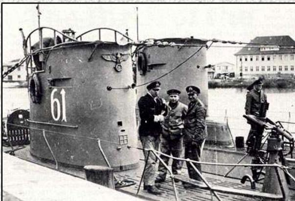
Left (C7): Here can be seen the tower of U 61, with the curved railings extending high above the tower bulwarks. Note the absence of the magnetic compass fairing compared with the unidentified IIC on the right. On U 61 the hatch at the front can be seen, as can the square and cross marker on the outer surface.
