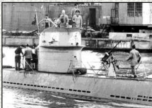
Above (D5): On the IICs there were 19 vents to the rear of the two dots. On a number of IIDs there were 18 vents, which is a useful point of differentiation. On U 149 and U 152 there were 17 to the rear of the two dots.
