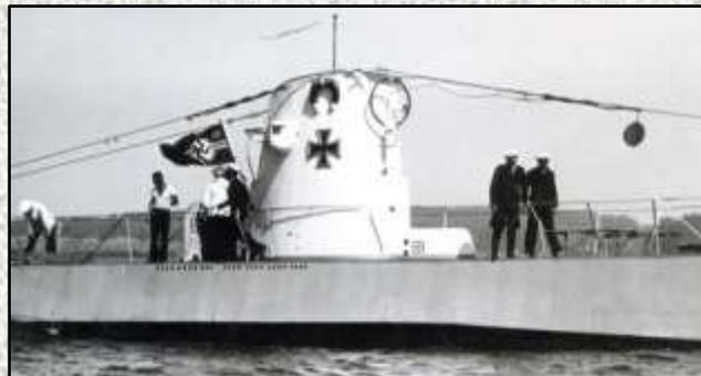
Below right (B14): On this drawing of U 7, note the large housing for the navigation lights (aft of the pre-war number 7). This bulky housing projected significantly out from the tower to allow the light to shine forwards without impediment.
