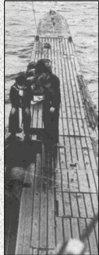
Above (5): The forward deck of U 826 shows the "planked deck" used on later VIICs and VIIC/41s. It can be seen that this style of deck was much simpler, requiring far fewer man hours to produce.
