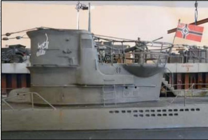
Left (54): Here can be seen the finished model from the port side. The reshaped trunks, plate at the front of the trunk, railings, ladder and grill at the top of the trunk can all be seen. The small group of ventilation holes above the rear of the trunk were added via a part within the custom brass sheet. They could have been drilled but experience has shown that a brass part produces a much neater result.
