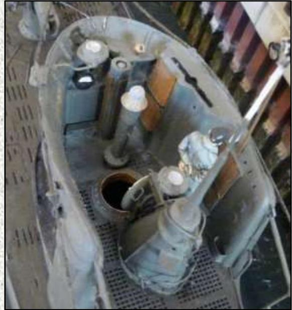
Above (58): Many details can be discerned in this photo. The two magnetic compass repeaters - one directly in front of the attack periscope housing and the other near the front of the tower - can be seen, Below the front repeater is a cable to the boat below and a black and white dial. Over the right hand side of the “dashboard” area is a brass voicepipe on a scratchbuilt shelf.
