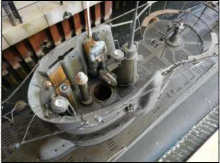
Above (57): A view of the D/F housing, which was completely rebuilt using plasticard. The brown areas are the wooden slats (again scratchbuilt in plasticard) with wooden extendable seats below.
