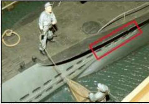
Left (51): The area within the red box shows the extra five vents replicated using photo-etched brass. This change is essential for modelling a VIIB rather than a VIIC. The black pieces above are the breakwaters, which helped to reduce water splashing up on the crewmen operating the 88mm deck gun.
